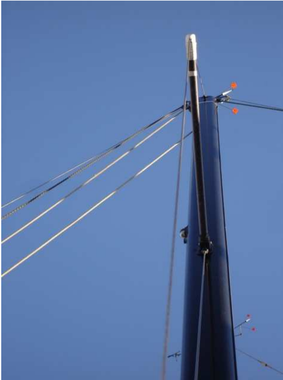
Install & Check shrouds
